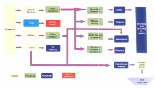
An inbuilt overhead magnetic band ensures automatic separation of ferrous component from the feed, whereas employees, wearing appropriate safety equipment such as gloves and helmets, stand by to physically separate other metals such as aluminium and copper from the moving conveyor belt. All plastic components are deposited at the end of the conveyor belt. These metals (aluminium, steel, copper) and plastics which are of high purity in nature are then usually sold to smelters.
